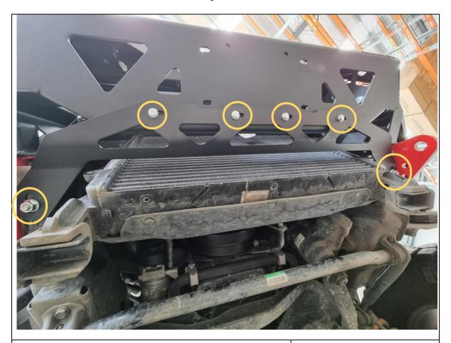
80. Install the tension strap connecting the bottom of the winch cradle to the previously installed M12 bolt plates, using 4x M18x20 hex bolts and heavy duty washers, and 2x M12 flange nuts.
