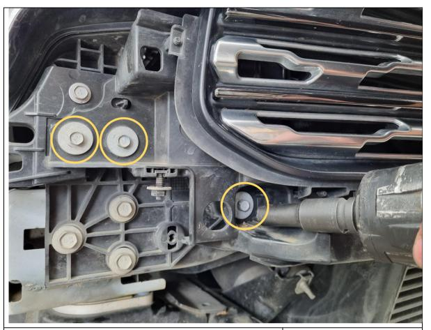
24. Remove the 6x 10mm hex bolts (3x per side) securing the bottom corner of the grille to the vehicle.
