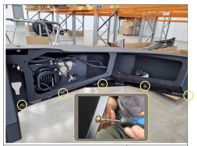
66. Fit 5x M6 cage nuts into the rectangular slots on the bottom of the bar wing.
