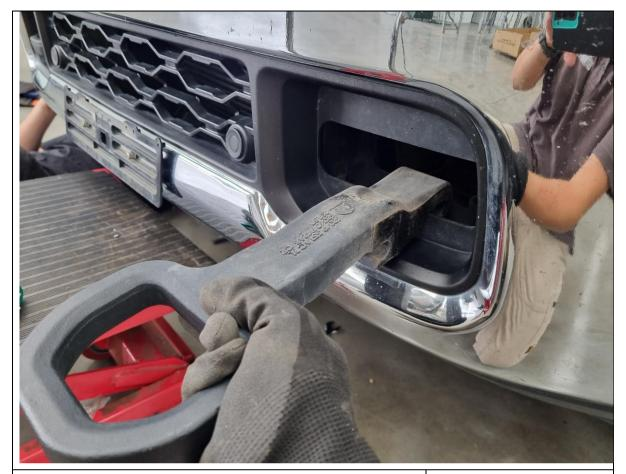
6. Pull out the loosened tow hooks through the opening in the front of the bumper.
