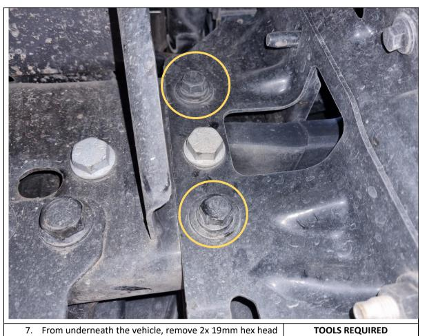
7. From underneath the vehicle, remove 2x 19mm hex head bolts securing the steel bumper to the chassis, per side.
