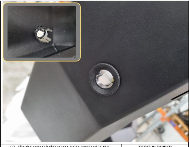
50. Clip the sensor holders into holes provided in the bulbar. Ensure their orientation matches the factory steel bumper.
