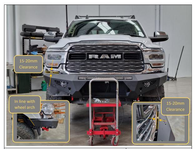
75. With assistance, from another person, align the bar with the edges of the vehicle. The bar should sit symmetric left/right on the vehicle.
