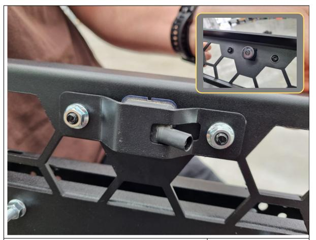
84. If relocating the front camera, sandwich/clamp the camera between the mesh fairlead mount and camera relocation bracket and secure using 2x M16x16 black button head bolts, black flat washers and flange nuts.
