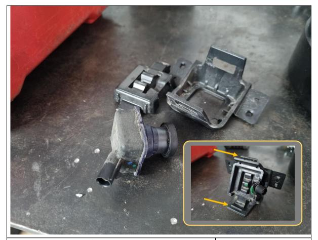
29. Unclip the camera from its plastic housing and set aside for later.
