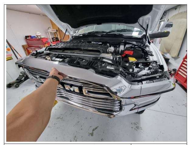
18. Remove the top chrome trim by pulling forwards and away from the vehicle. Set aside for reassembly.
