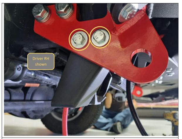
89. Fit the bash plate mounts to the tow points and secure with 2x M10x40mm hex bolts, flat washers and flange nuts (each).
