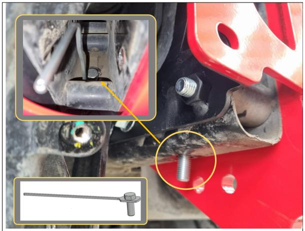
38. Install 1x M12 lollipop bolt plate through the bottom hole in the chassis rail, per side. Leave hanging for now.
