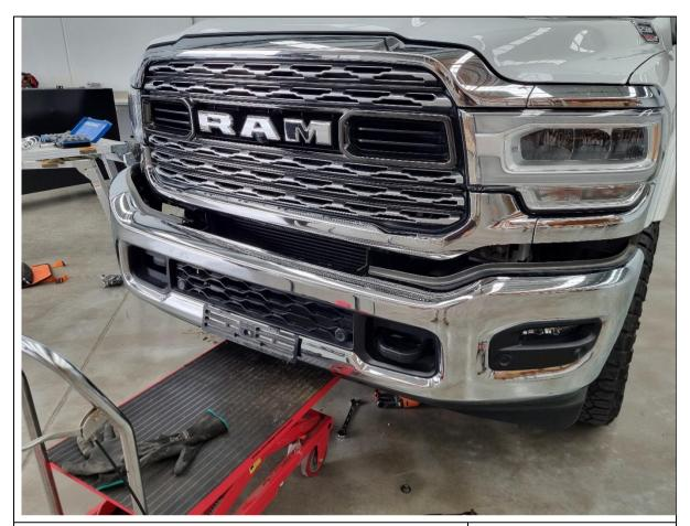
8. Pull the bumper off the vehicle and set aside in a safe place.
