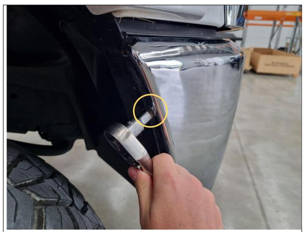
2. Remove 1x 10mm hex bolt securing the inner wheel guard to the bumper, on each side.
